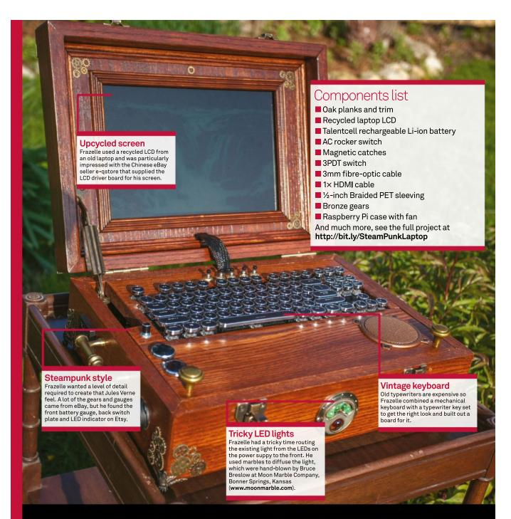
Right At its heart is the Pi 3. Almost every cable was shortened in the box. Frazelle had to open up the PSU to route the power switch to one on the back of the box.
